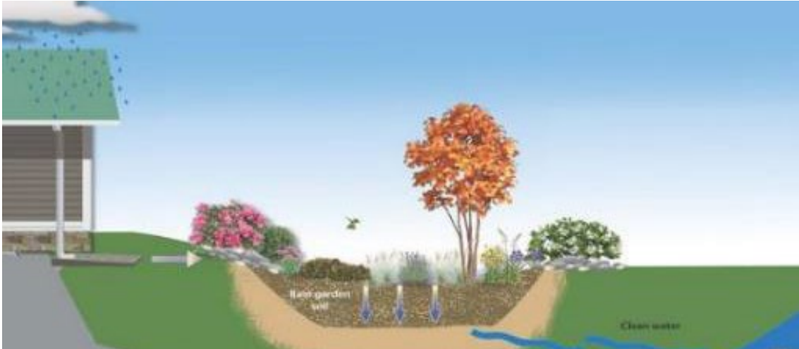
Example of rain garden (Source: United States Environmental Protection Agency)
